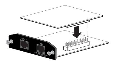
Figure 36. Installing DIMs
